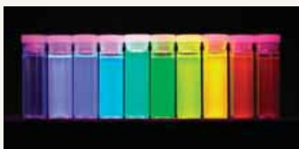
Quantum dots of the same material of different sizes emit different characteristic wavelengths
